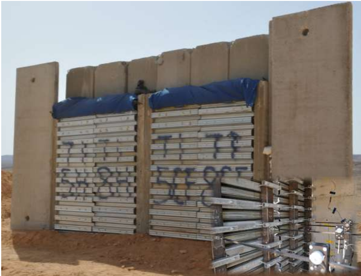
Figure 36 HSS target before test
