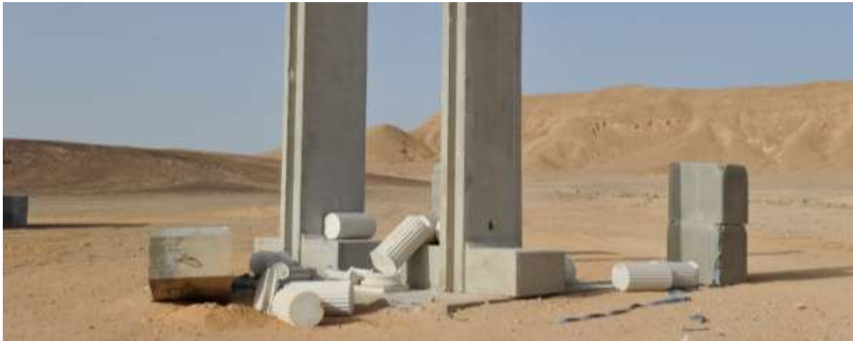
Figure 32 Neoclassical multi-drum columns after test
