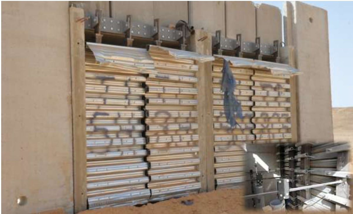
Figure 40 HSS target after test
