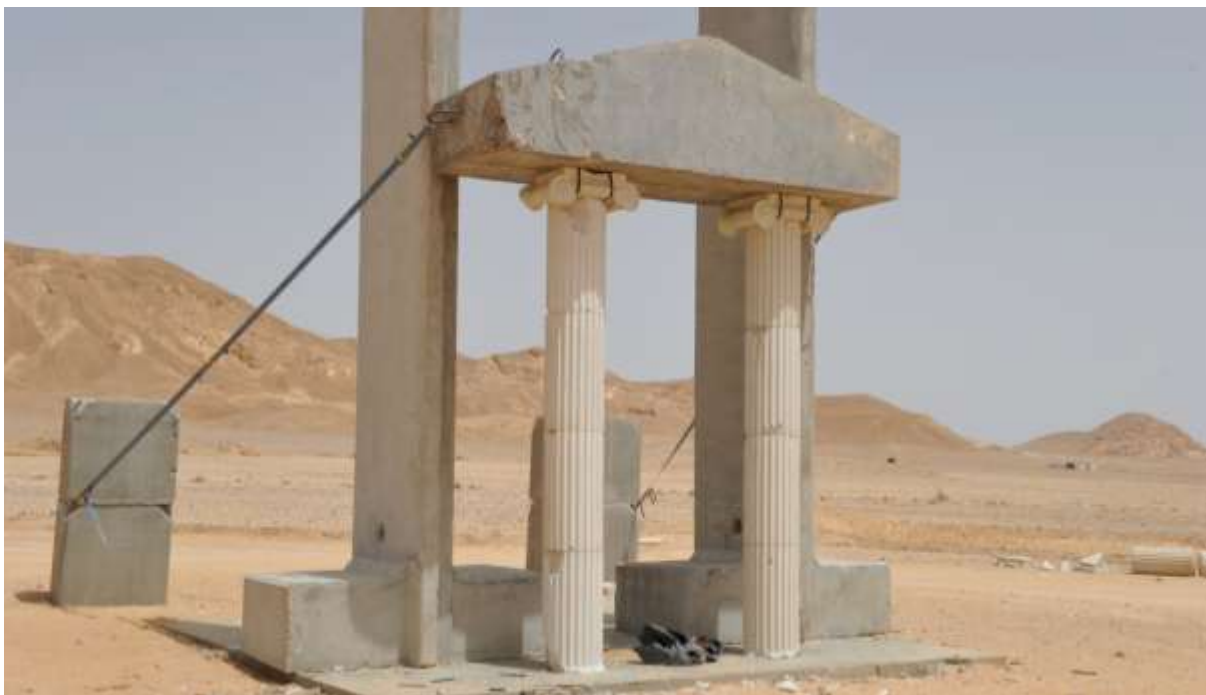
Figure 47 Neoclassical multi-drum columns before test
