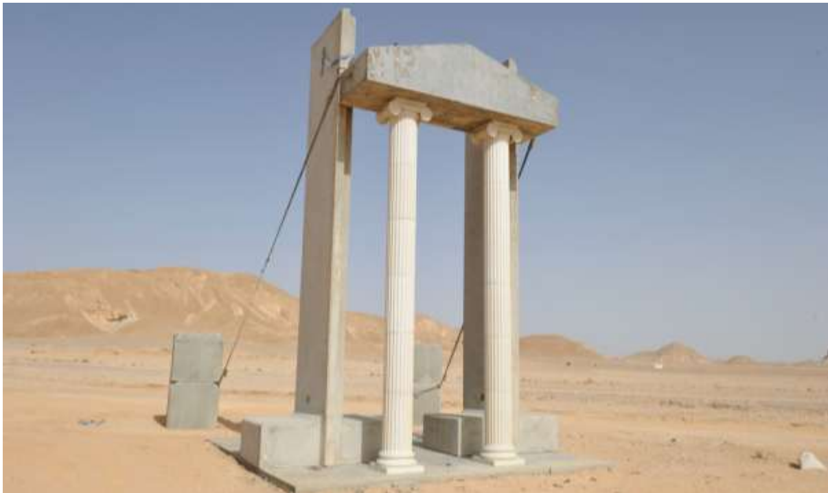
Figure 31 Neoclassical multi-drum columns before test
