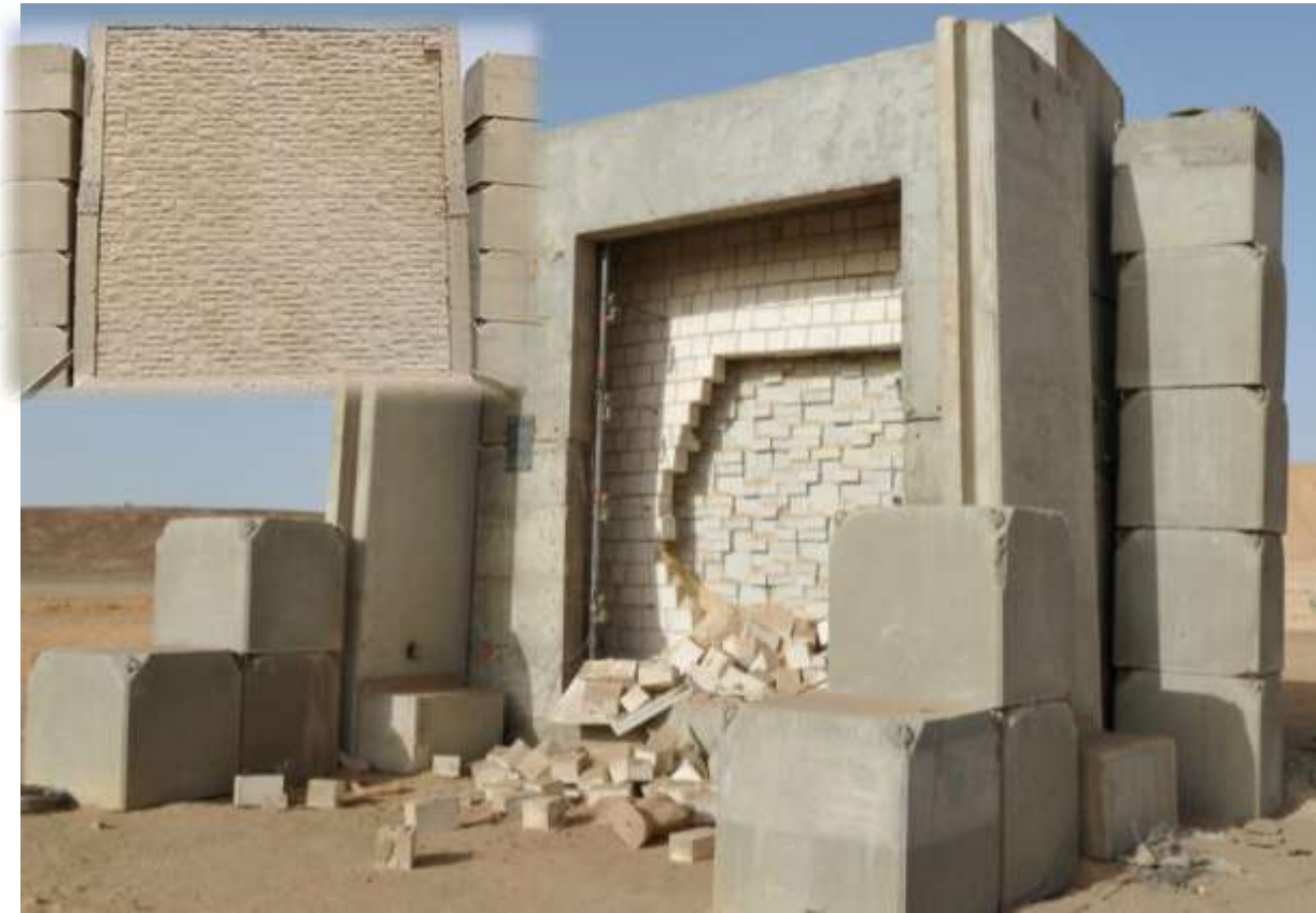
Figure 34 Historic masonry wall after test
