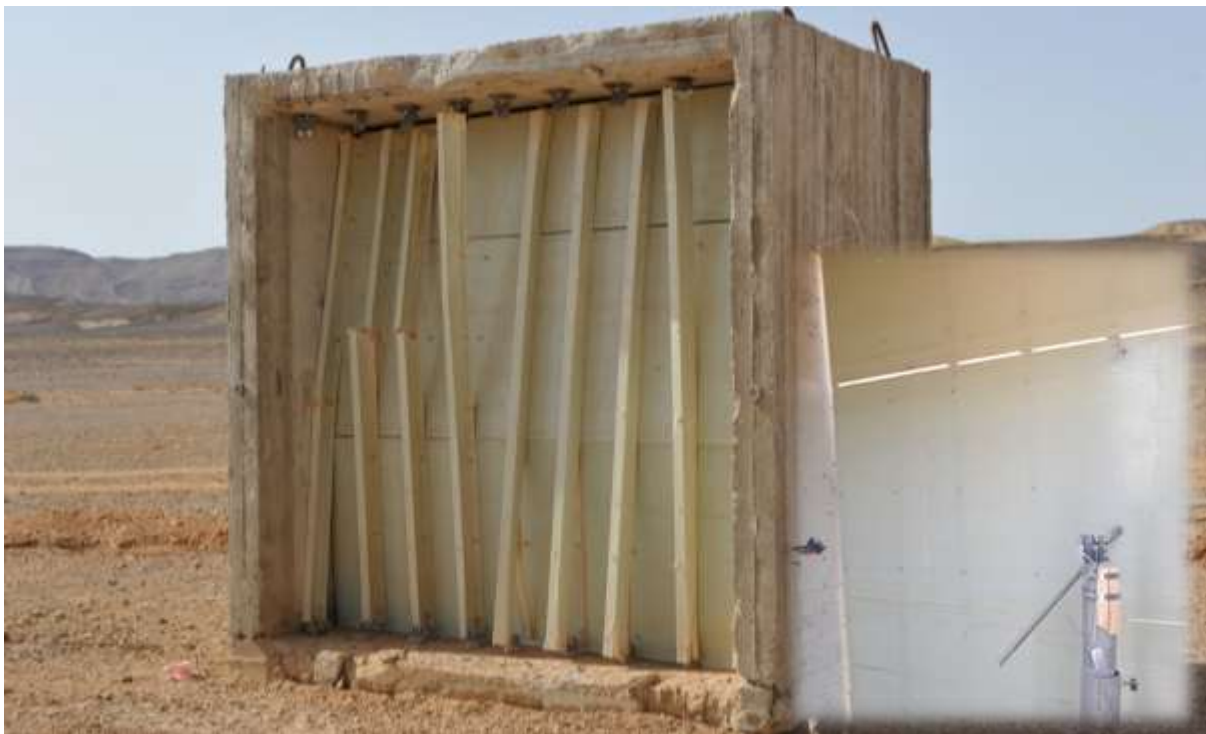
Figure 43 Fibre reinforced plastic element wall after test
