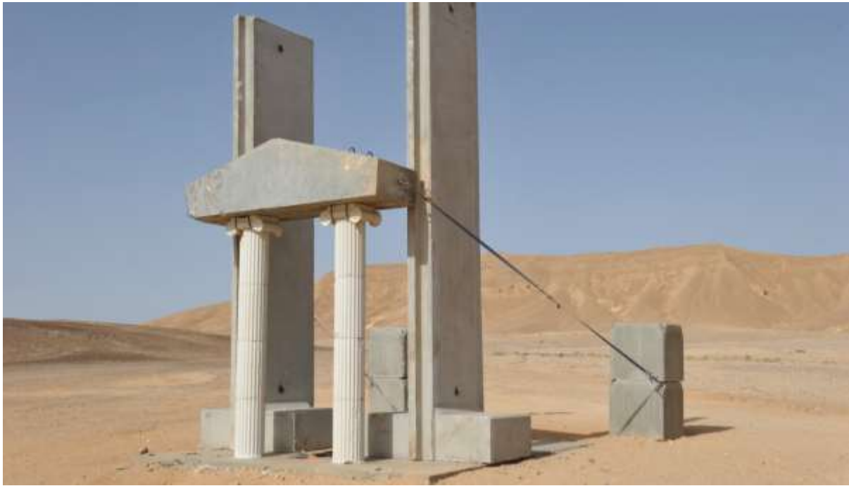
Figure 38 Neoclassical multi-drum columns before test
