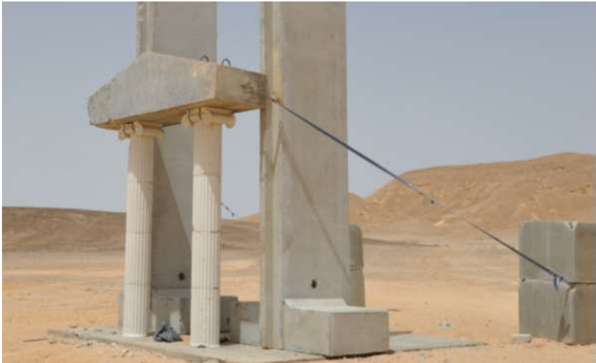
Figure 50 Neoclassical multi-drum columns after test
