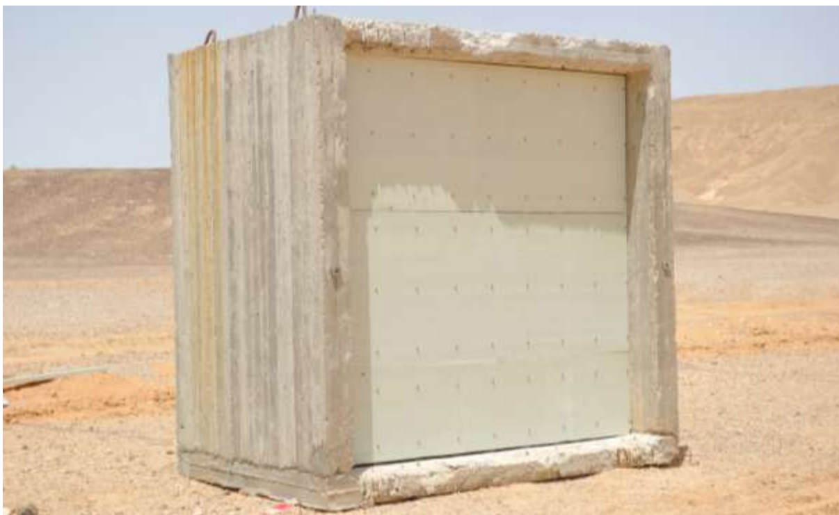
Figure 39 Fibre reinforced plastic element wall before test
